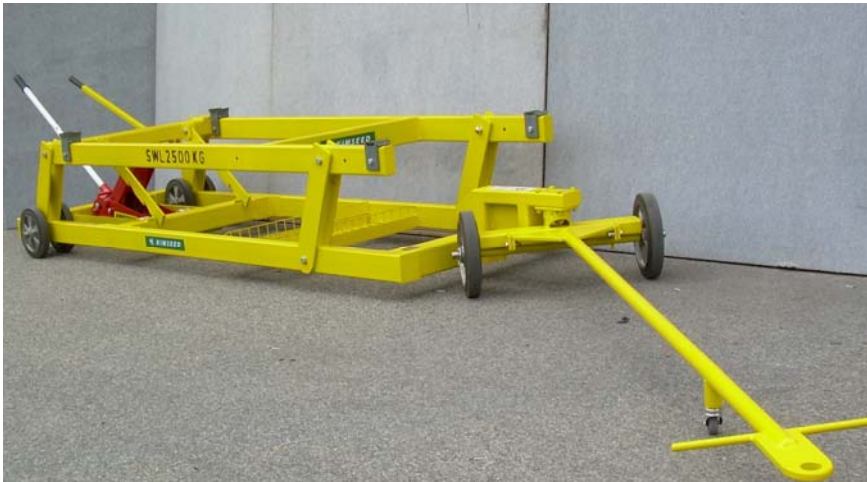
Heavy Duty – Multi Helicopter (206-206L & 407) Ground Handling Trolley
