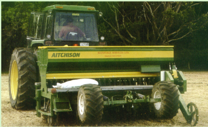
Minimum penetration Drill with all the weight on the press wheels
