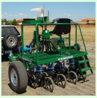
The Kimseed Combi-Cone Seeder has been designed to suit linkage tractors or be towed by tractors or large 4WD vehicles. The Disc type plot seeders are used by Agricultural Departments, Universities, Plant Breeding Research contractors in Australia and overseas.
