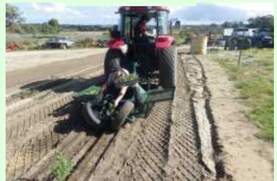
Tree Planter – tractor drawn (above) Coulter wheel and ripper (Below)
