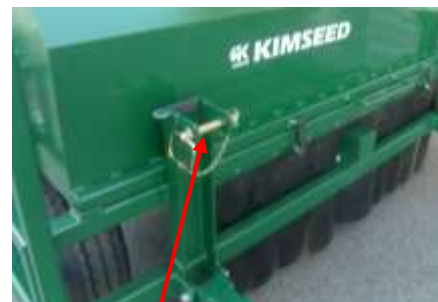
Pin in Transport Brackets when machine is operating with harrows down.
