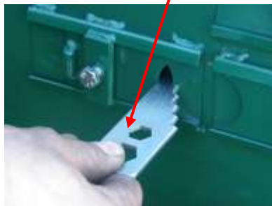
Drum key to set outlets evenly.
