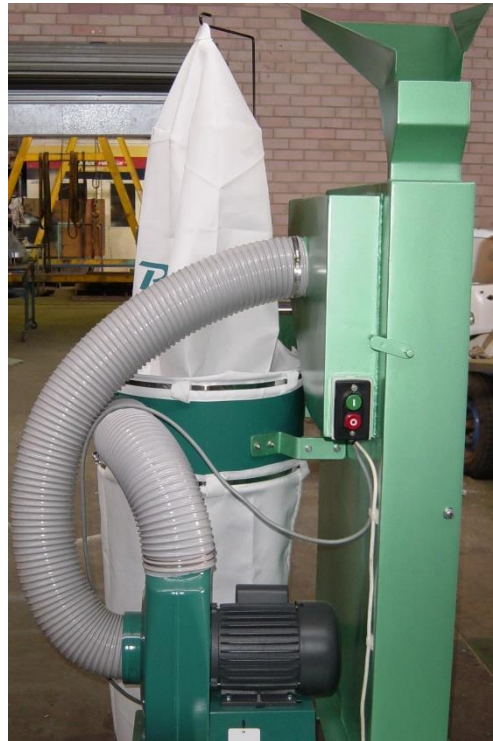
Suction fan and dust control system.
